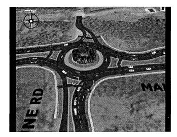
The Roundabout at Barrydowne is designed to allow about 3 cars from the Garson West-bound lane to "be on hold" waiting their turn to cross the East-bound lanes in the Roundabout to exit the Roundabout and travel South-bound on Barrydowne Road. Problem is, a steady stream of East-bound traffic in the curb lane, coming from Notre-Dame, is simultaneously using the Roundabout to access
