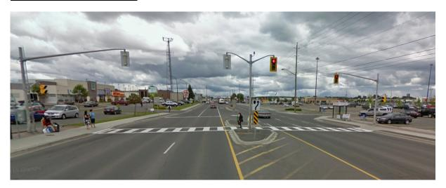
Pedestrian traffic signals manage the interaction between pedestrians and vehicles, and present operational benefits to pedestrians by providing priority over vehicles at all times. This priority may provide a sense of security for pedestrians, encourage pedestrians to cross at the controlled location and limit the number of locations where pedestrian crossings occur.
