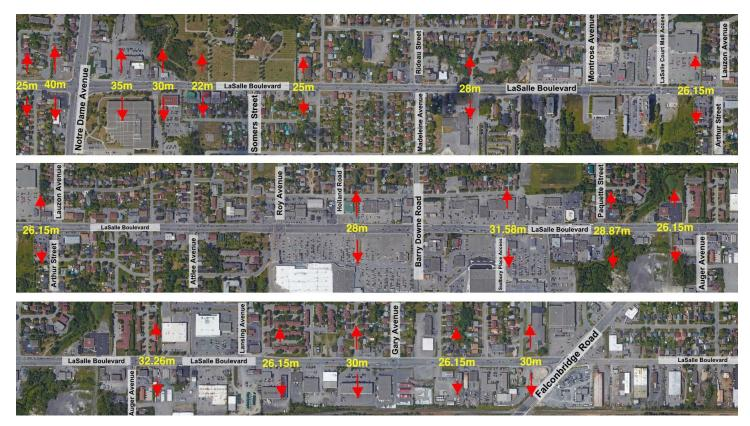
Figure 5: Right-of-Way (ROW) Widths
